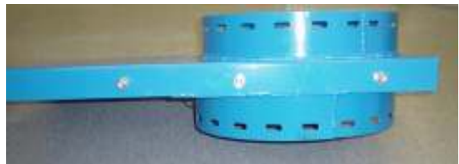
Side view 17" 1/4" dia. ring into bin bottom Larger diameter ring down
